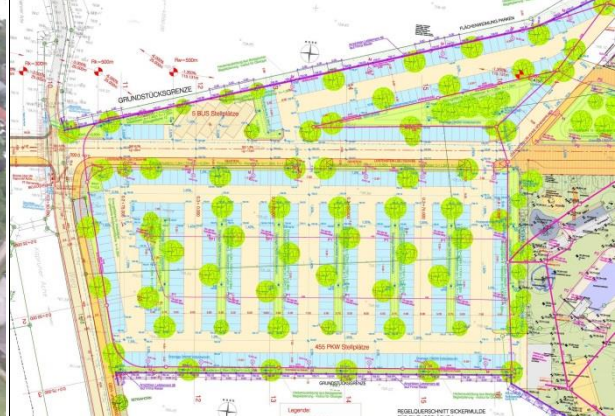
Detail design of parking area, dewatering design
